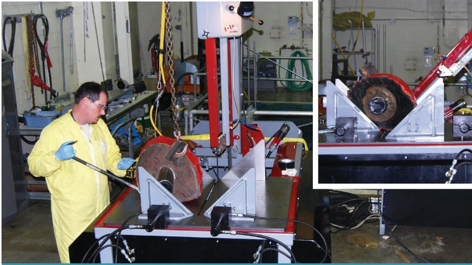
Sectioning control rod drive mechanism nozzle and surrounding reactor vessel head material on large capacity vertical band saw. Blade angle range is  $\pm 45^\circ$  (inset)
