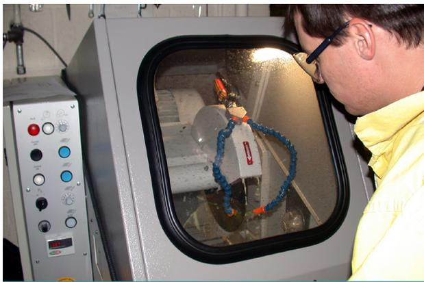
*Precision abrasive cut-off saw*
