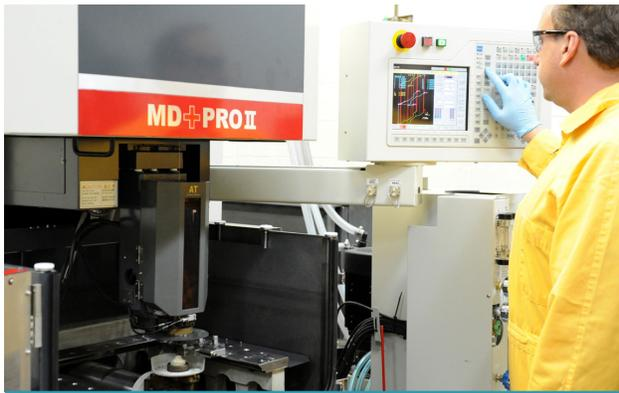
*CNC electrical discharge milling machine*
