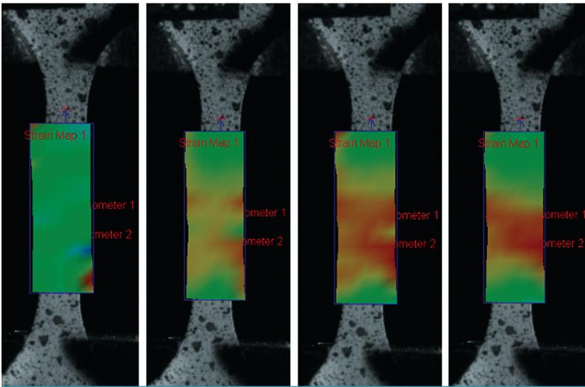
Strain mapping using DIC system
