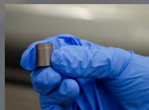
In Toronto, we manufacture ceramic pellets from natural uranium dioxide powder. After pressing, baking, grinding and inspecting the pellets, we send them to our Peterborough facility where they are placed in CANDU® fuel bundles. The fuel bundles are then sent to Ontario Power Generation's Darlington and Pickering Nuclear Generating Stations. Both our Peterborough and Toronto facilities are licenced by Canada's nuclear regulator, the Canadian Nuclear Safety Commission (CNSC).
