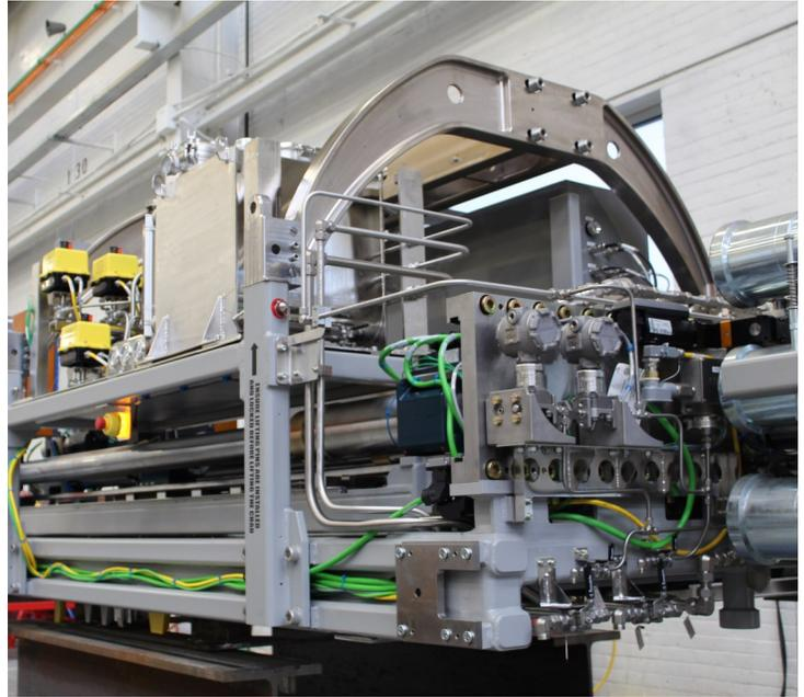
*The second Bruce Reactor Inspection Maintenance System (BRIMS II) nears completion in February, 2017. BRIMS II, like its predecessor BRIMS, is a remote-controlled machine, about the size of a small car, featuring an assortment of interchangeable drives used to deliver critical inspection and maintenance tools to the nuclear reactor fuel channels.*
